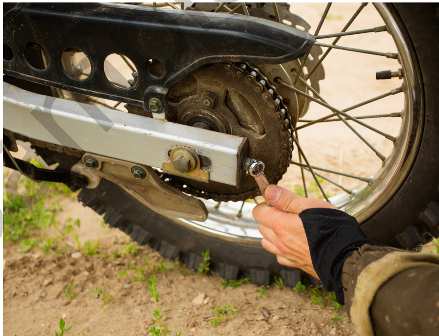
Adjusting the chain is an important part of the post ride check.
