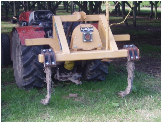
Image 57: Ripper attached to the back of a tractor, used to help improve soil drainage (Shane Max).
