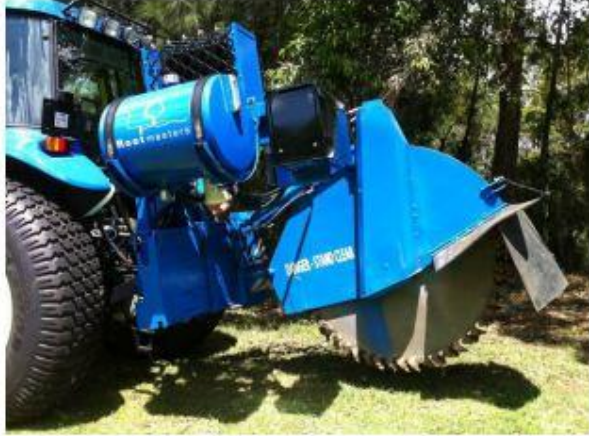
Image 56: Root pruning is done with a large blade attached to the back of a tractor that drives slowly down the rows and cuts down into the soil.
