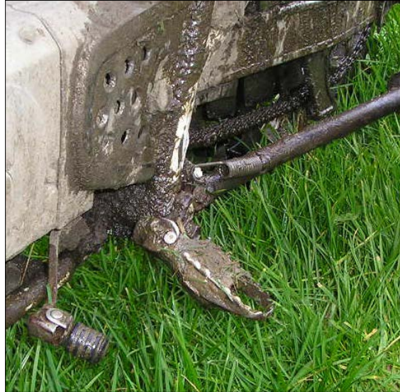
A common fault on farm bikes is bent foot pegs. This is a hazard, as your foot will slip off the peg very easily
