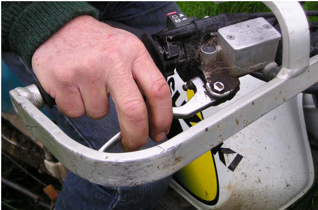
Lever is well adjusted. Rider can operate with two fingers allowing a good grip on the handlebars.
