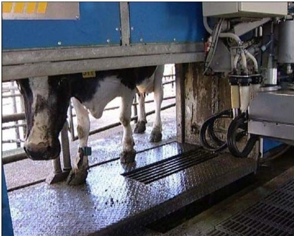
Figure 20 A cow enters a robotic milking stall
