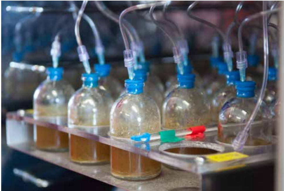
Figure 4.1 One of the mitigation options covered in this report is the use of chemical compounds that inhibit the production of methane in the rumen. The photograph shows the testing of potential methane inhibitors in rumen fluid at AgResearch in Palmerston North.
