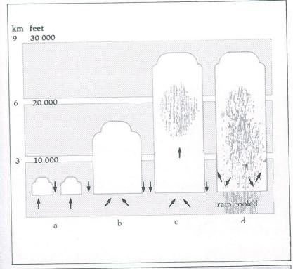
Heat is transported upwards; cloud forms when the air reaches condensation level (a). Latent heat derived from condensation helps keep the air buoyant and it continues upwards (b), forming deep shower clouds in which raindrops first form at upper levels (c), and later reach the ground (d)
