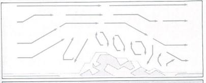
When it crosses hilly terrain the air flow becomes turbulent. The turbulence is caused by the presence of uneven terrain and the increased frictional drag
