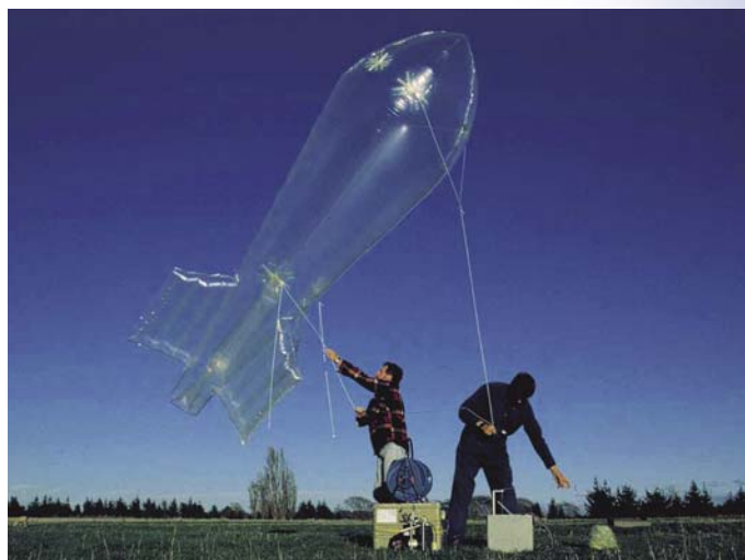
Launching a tethered kytoon to carry aloft instruments to measure wind speed and direction, temperature, and dew point and tubing for collecting samples.
